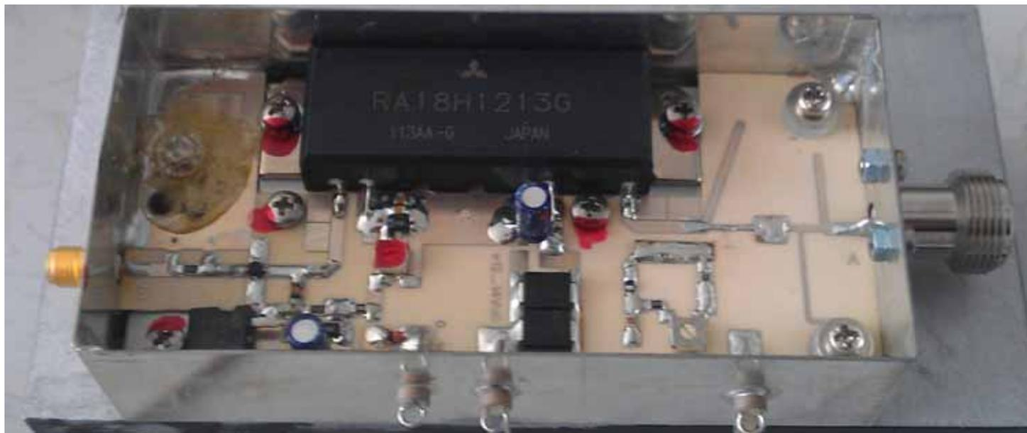
Replacement 12 volt 23cm 20 watt PA, made by DG0VE from Germany, mounted on a heatsink ↑
