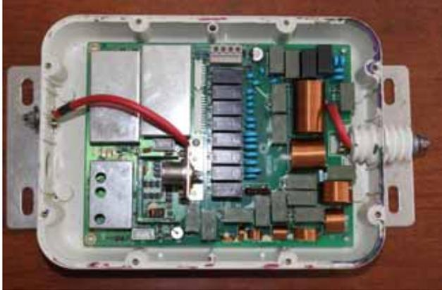
Relay with jumper wires removed ↓
