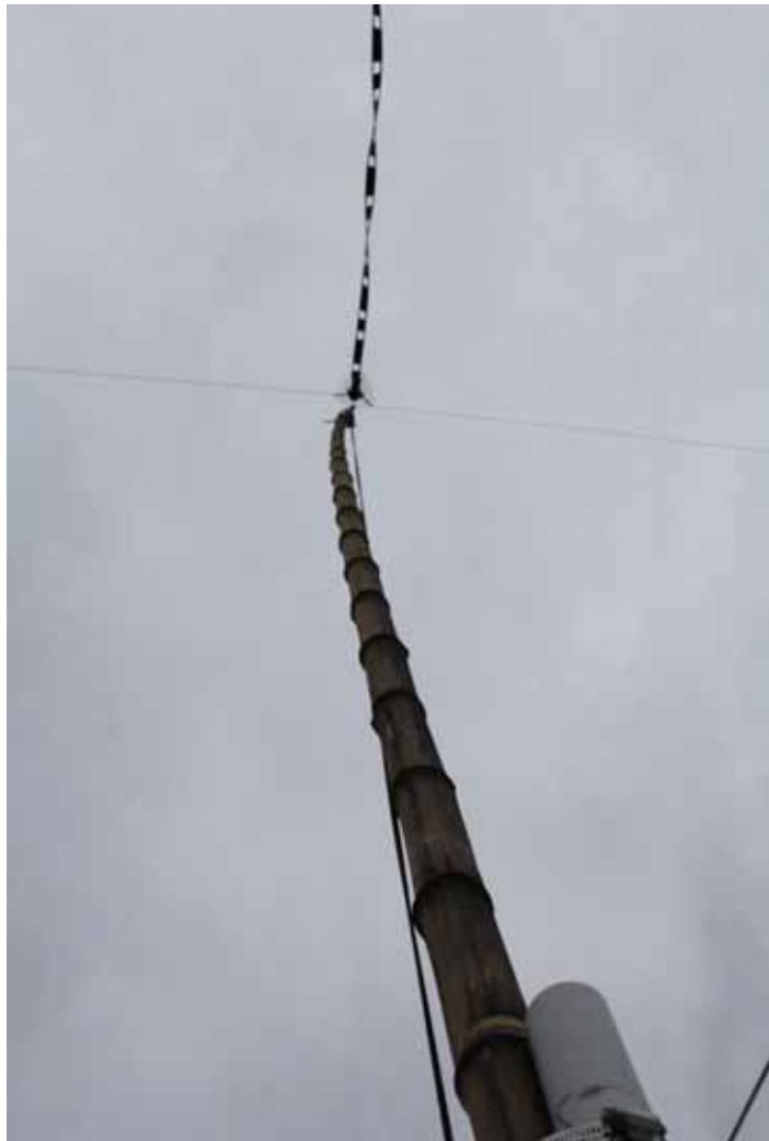
160 top loaded antenna, with ground radials over the rooftop, with the inverted 'V' to the left and looking up at the feed to the 'V'. As well as the three guys to adjust the capacity hat radials, another dedicated three guys were put so no need to lower the mast when making tuning adjustments, plus support in high winds. Three guys are set lower down the mast to stop it oscillating in the winds.
