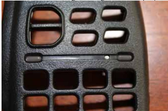
The enlarged audio hole, with the drill used ↓
