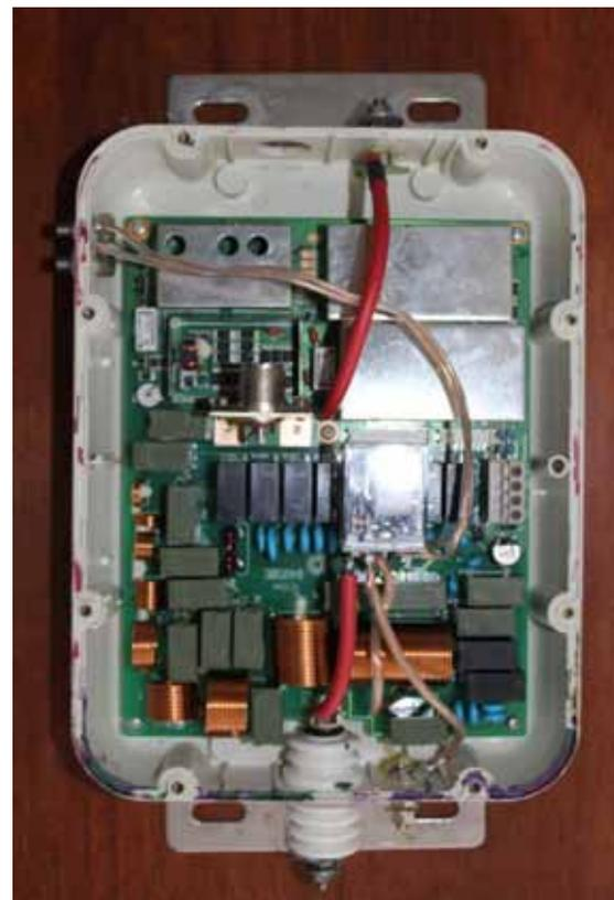
← Completed AH-4 with relay inside, relay held in place with a dab of glue
