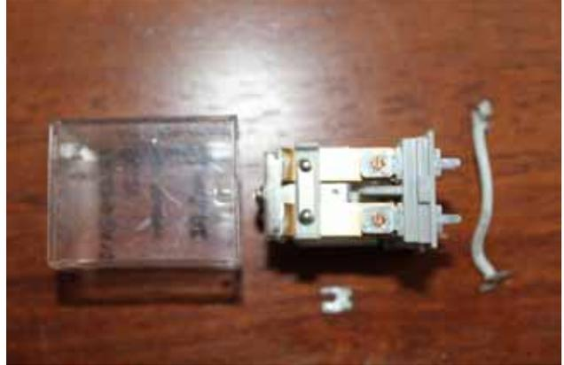
Relay contact pairs bridged with solder via a copper strip ↓
