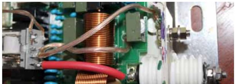
Close up of the new relay switching of the HF ↑
