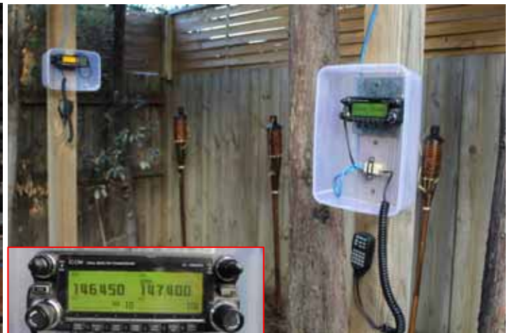
23cm ID-1 (yellow screen) and the IC2028H (green screen) Microphones coil inside boxes when not in use. ↑
