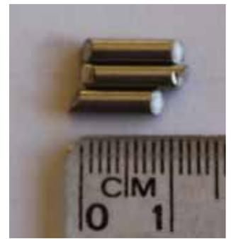
40 meter stainless steel is so hard that bolt cutters were used to cut it to tune, the pliers and hacksaw did not make a mark on the steel. Three bits cut off and resonance tested until VSWR was OK → Each piece removed brought centre frequency up around 50kHz, so >150kHz needed to set it up.
