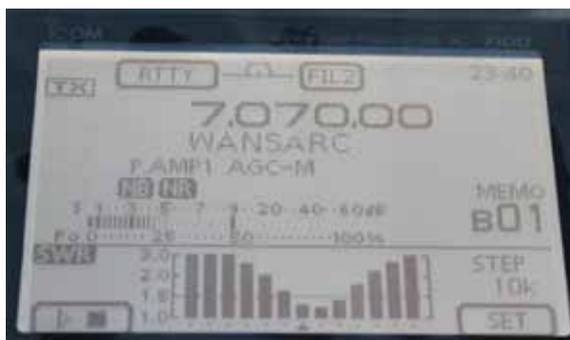
Sweep of 40 meter whip, ▲ is centre frequency, (each bar contains highest VSWR in its 10kHz sample range) 7055 to 7100 low VSWR, as FG01 Analyser said ↑ Actual usable range of 40 meter whip is 7040kHz to 7120kHz, if you 'allow' VSWR up to 2:1, then its another 50kHz either side.
