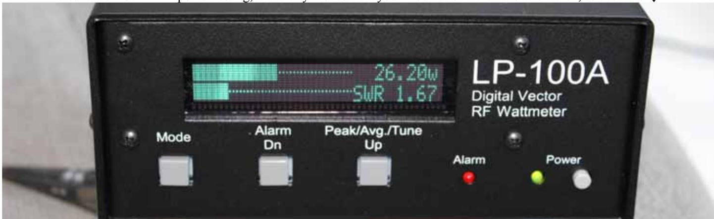
Above is actual AM carrier into the 40 meter whip on the car at 7070kHz, where along with my other tests is centre tune ↑
