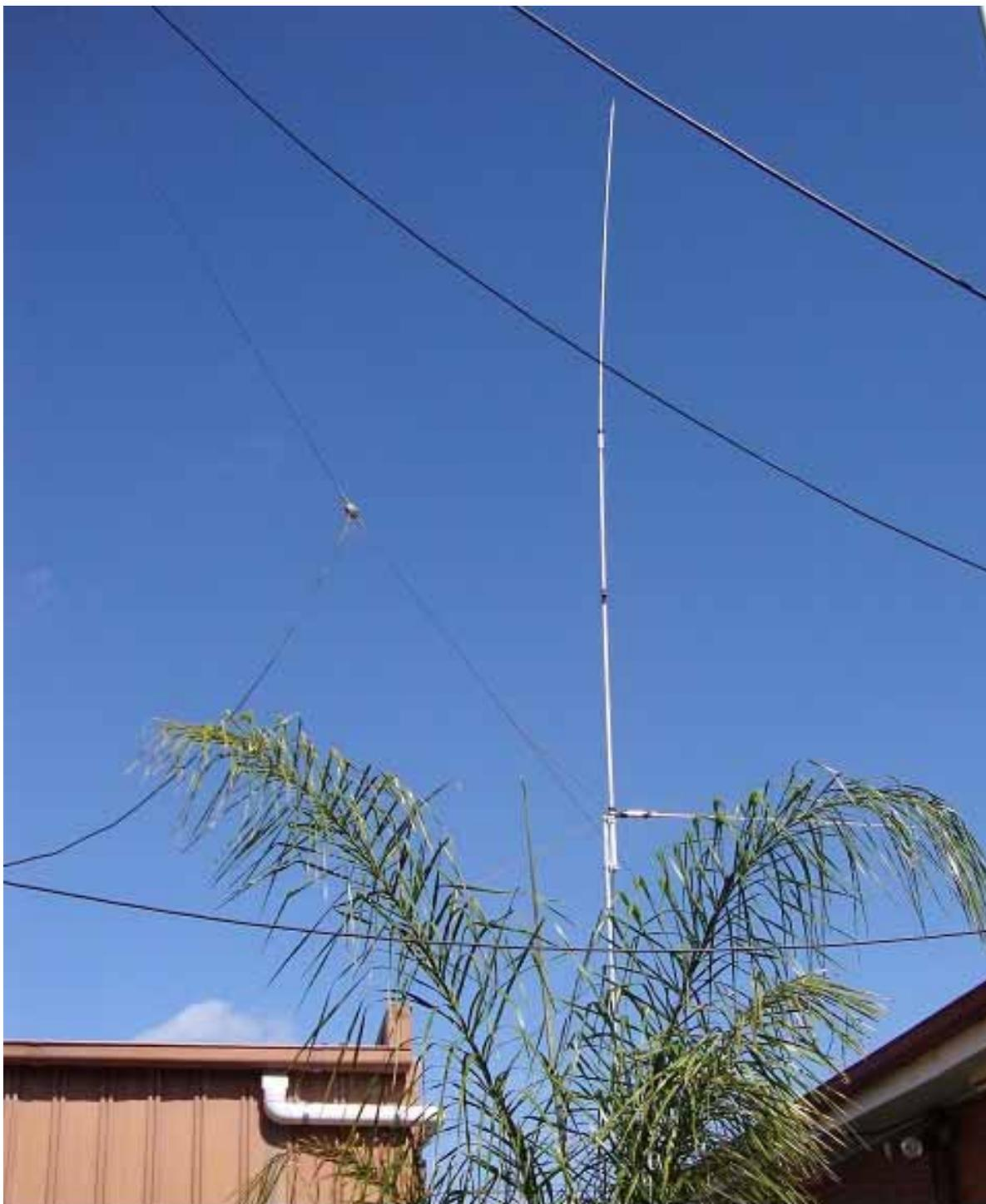
The 10m sloper was looking a bit sloppy DX wise so the opportunity rose to co-buy with Frank VK3OP a high gain vertical for 10m and 6m. The CP6-10 is a single 5/8 on 10m and 2x 5/8 on 6m, providing 3.4 dB and 5.5 dB respectively.
