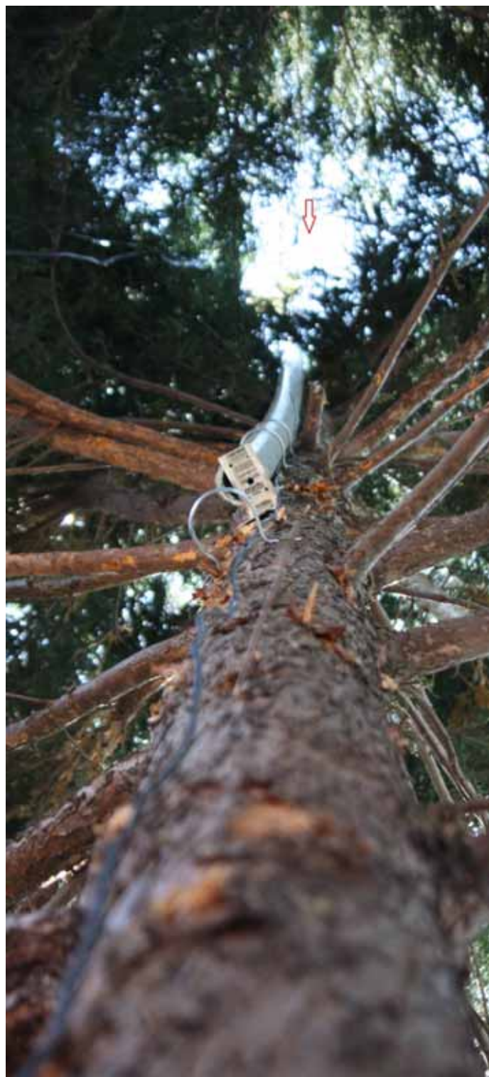
The mast up the tree with AH-4 indicated by red arrow ↑ Black "ground side" wire is visible, the end is 1.5 meters above the ground. This will stop the rabbit getting zapped with RF.
