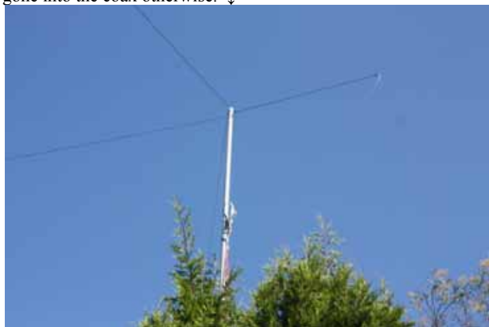
Coax feed point, all covered in sealant. ↓ (since removed)
