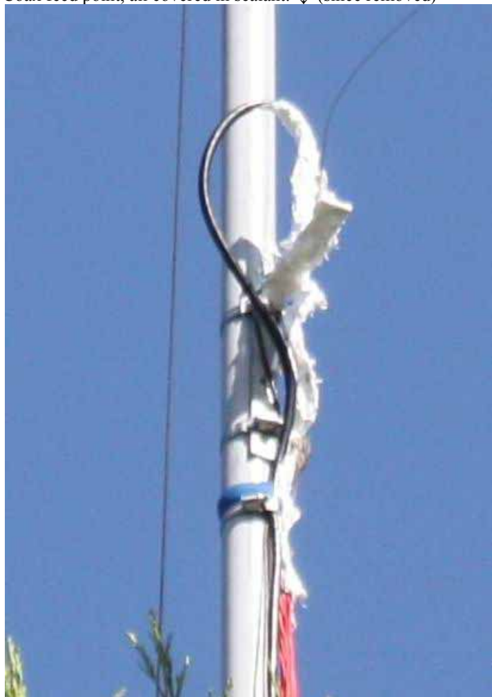
Coax feed point, all covered in sealant. ↓ (since removed)
