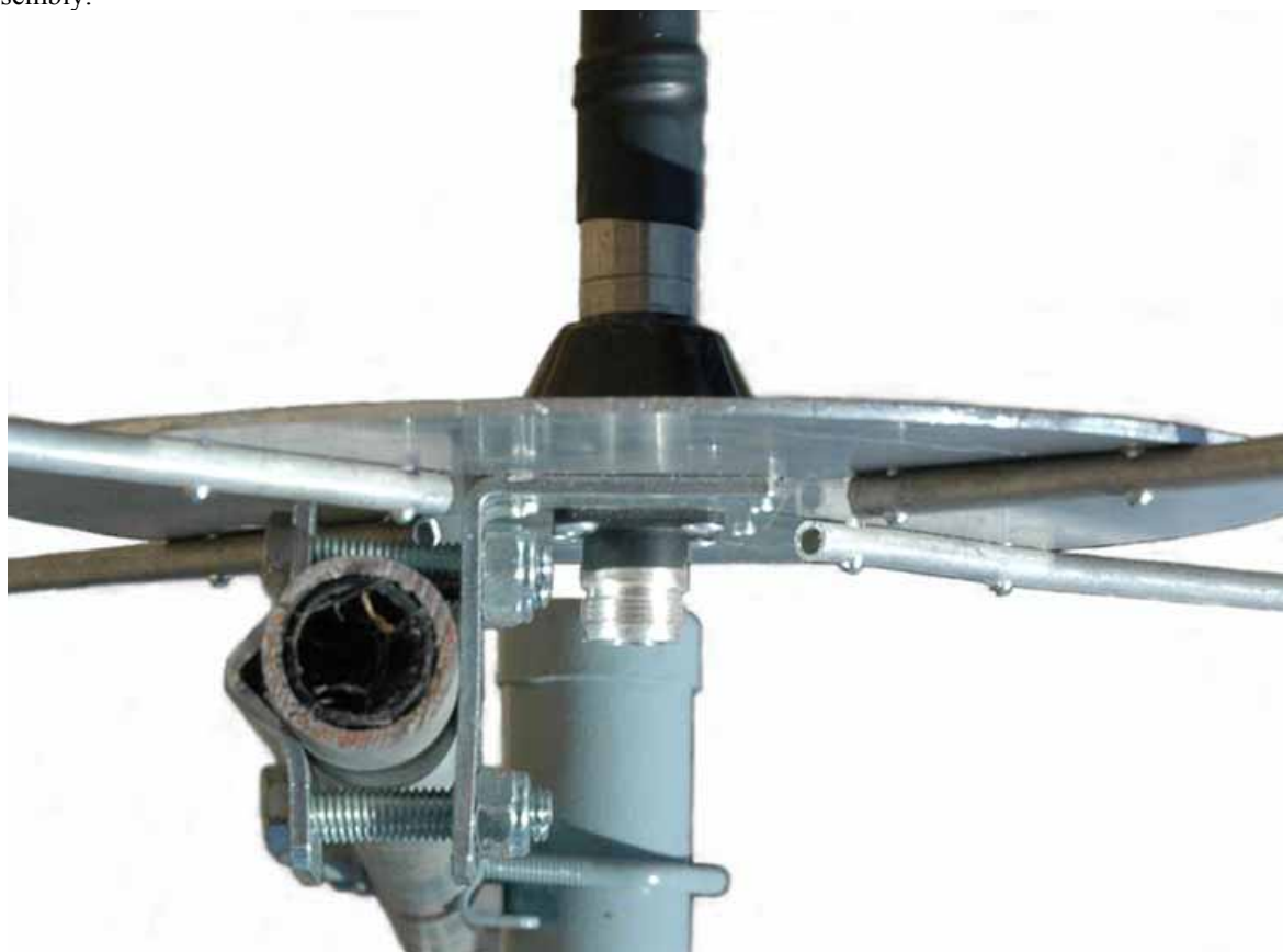
Photo 4 Standard mobile antenna mount adapted to the ground plane assembly - Side view
