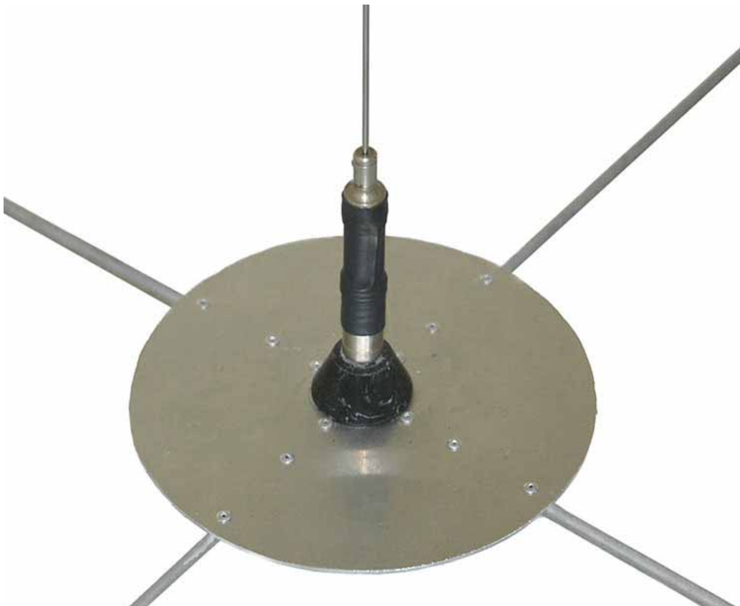
Photo 3 Standard mobile antenna mount adapted to the ground plane assembly - Top view
