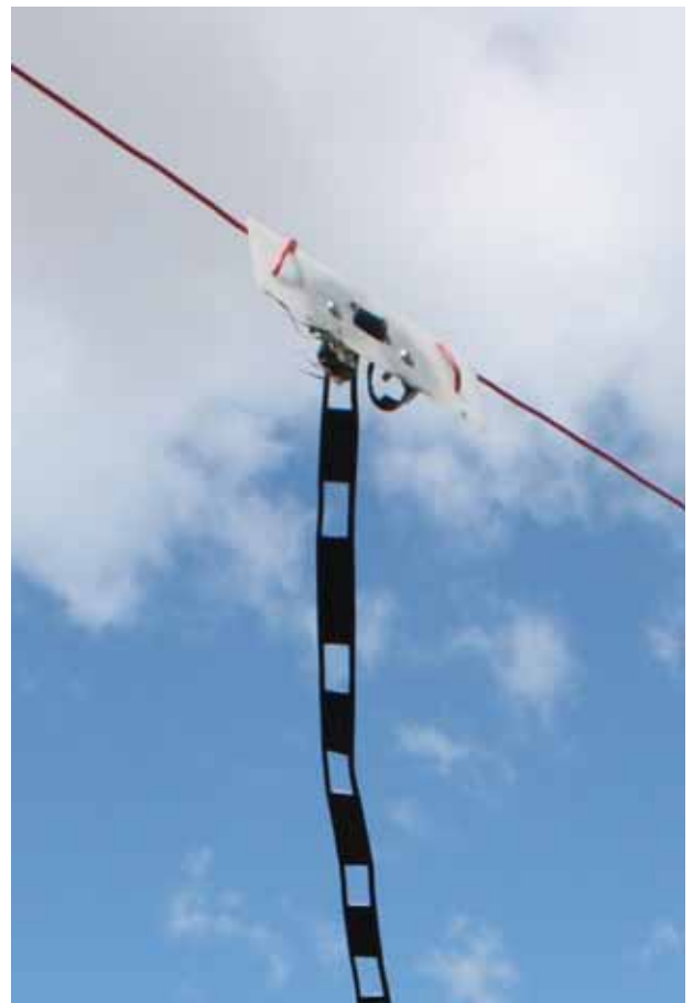
The ladder line to the end fed Zepp ↑
