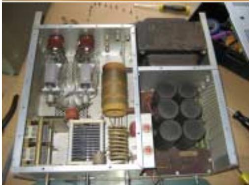
Now safely back in Australia, I unpacked my new/old toy and very carefully fired it up into a dummy load. With 50W drive it produced 350W PEP output, with 75W drive it produced 450W PEP. Not bad for a completely original 37 year old amp with no components replaced, apart from the tubes. Some of the capacitors in the power supply were looking a little sick, so I decided to restore it to its former glory.
