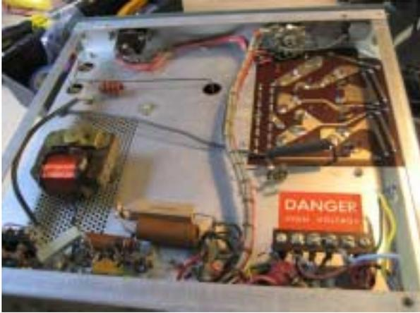
This one-ohm resistor replaces the solid wire jumper from the RF choke AN to the 1000pf "door knob" capacitor at AP. The new suppressor assembly starts working at just above the 10 meter band. It actually has some effect on power output at 10 meters. You will probably notice a slight output drop at 10 meters from what you have come to expect.
