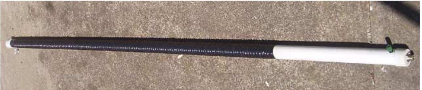
*the antenna and a couple of PVC cap fittings for the ends so that I could attach terminals etc. The first 70 feet of insulated wire was obtained at Jaycar at \$4.50 for a 25mtr roll. The other 70 feet for the 'long wire' portion of the antenna was made up of some odd lengths of "Figure 8" wire (from my scrap box) which I split and joined to make up the length and a visit to the local DIY store to get some PVC tube and cap fittings completed the shopping list .*
