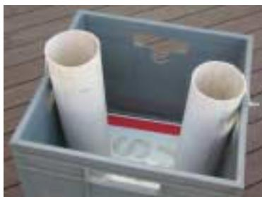
Sick of trying to sort your mobile whip antennae? Here is a simple solution using an old plastic crate. If you have an odd length of PVC pipe cut the pipe into lengths to suit the size of your whips (UHF or VHF). Cable tie your pipes to the side of the plastic crate and insert your whips into the most appropriate pipe. Jobs right.....Mark VK3PI
