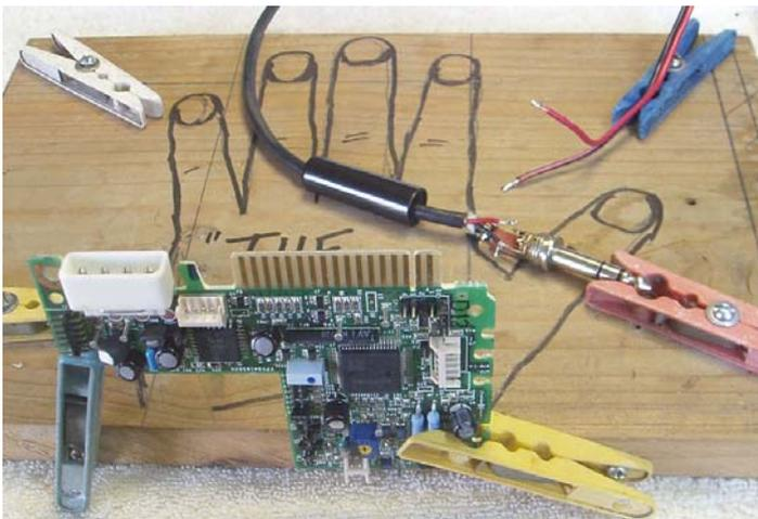
Picture of my ‘Third Hand’ showing some possible uses for it with the addition of a couple of extra pegs on the front edge to hold circuit boards vertically.
